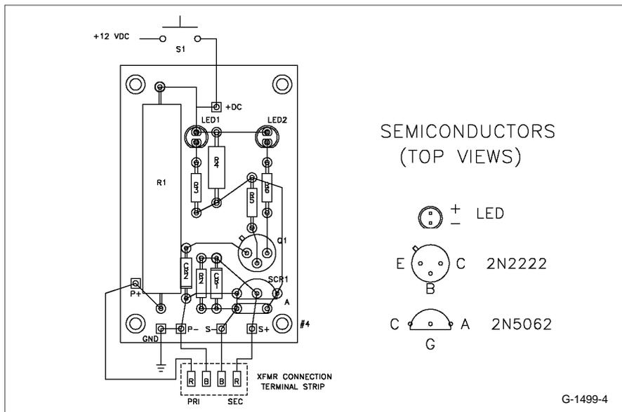
FIGURE 4: Components layout.
